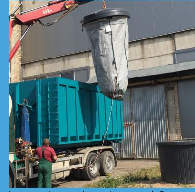
• Glass bag - bag that is used for glass. It is a two-layer bag, where outer layer of the bag is made out of polypropylene fabric and inner layer from PVC material.
