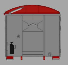
Using fireplug located on the front wall of the container, extinguishing water is supplied to the container. Moreover, after the battery is cooled down and temperature in the battery is below the critical ignition temperature, different valve located also on the front wall was designed to pump hazard water out from the container, for example, into hazard material tank.
